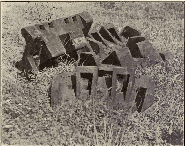
Fig. 89. Wear Plates with Lugs for Upper Tumbler.
