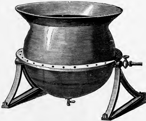
FIG. 19.—Steam-heated pan for boiling starch.
