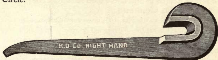
Fig. 110—Tool Wrenches like the above are used. The method of using the Wrenches is shown in the illustration on page 138.
