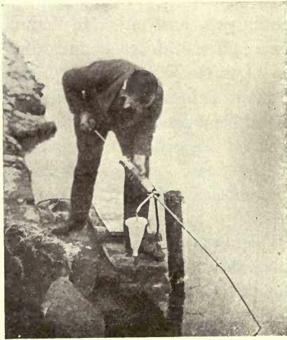
FIG. 9.—Plankton Pump. After Wilhelmi.
