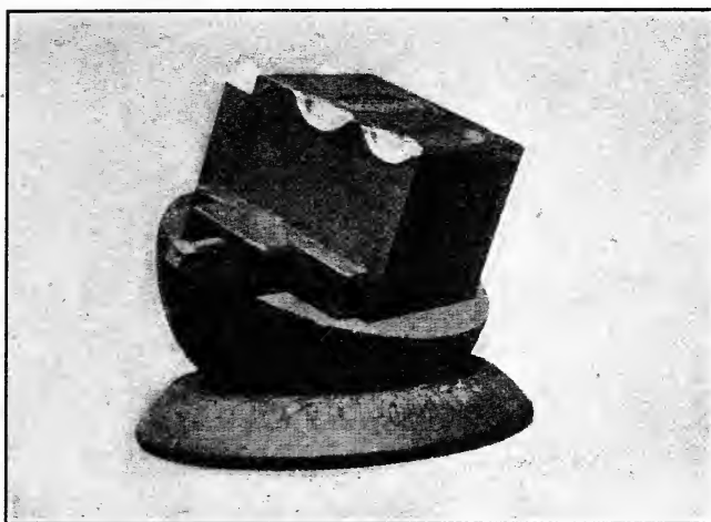
FIG. 5.—Special "Ball Vise" used in sinking drop-forging dies.
