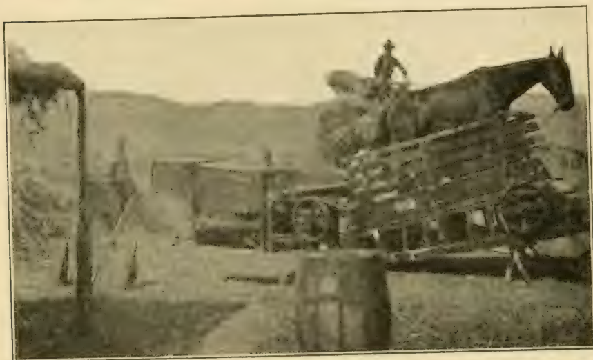
FIG. 100. Using treadmill for threshing grain from small plants on one of the Utah experimental dry-farms.
