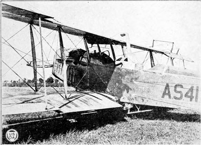
FIG. 3.—Air-suction hopper installed in Curtiss plane. Lid of hopper open for filling. Outlet for dust discharge is shown projecting below fuselage, together with a portion of lever arrangement for controlling the feed valve.
