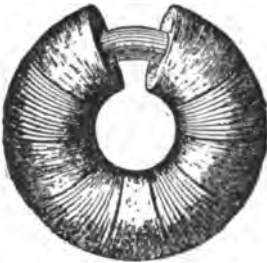
FIG. 486.—RING TRANSFORMER, WITH SANDWICHED COILS.
