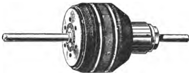
FIG. 842.—ARMATURE OF CROCKER-WHEELER MOTOR.
