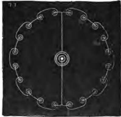
FIG. 414. CONNECTIONS OF FERRANTI ARMATURE.
