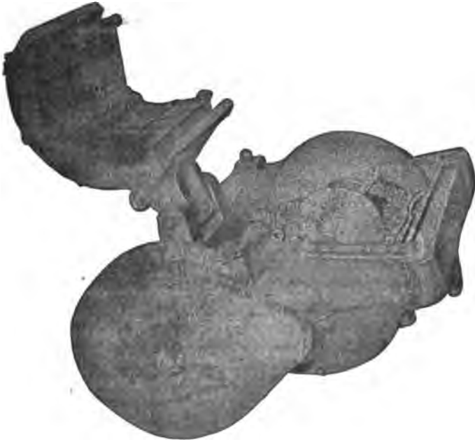
FIG. 346. —MAGNETS FOR STREET-CAR MOTOR.
