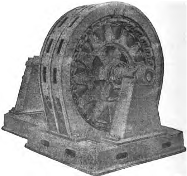
FIG. 428.—TWO-PHASE ALTERNATOR (225 KILOWATT).
