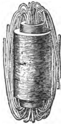
FIG. 487.—VARLEY'S CLOSED- CIRCUIT TRANSFORMER.
