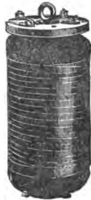
FIG. 498. SWINBURNE'S HEDGEHOG TRANSFORMER.
