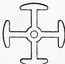
Fig. 9.—Double Shuttle or Walker Armature.
