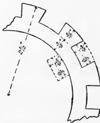
Fig. 86.—Side View of Cog-ring Armature.
