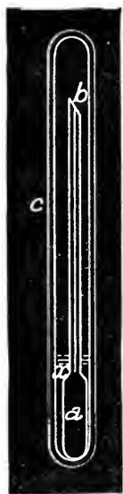
Fig. 22.—SPECIAL THERMOMETER FOR USE IN DEEP BORINGS.
