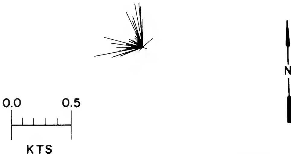
Figure 52.—Histogram of current velocities measured at 10 m during a period of 200 minutes on station 50, WEBSEC-70, 9 October 1970. Vectors are directed away from the apex of the array. Record was digitized at 3.5-minute intervals.
