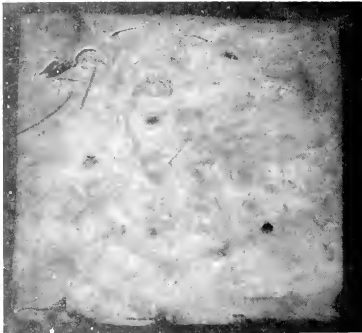
Figure 7b. —Radiograph of 1-cm thick slab of box core from station 9. Note abundant bioturbation and occasional pebbles. The distance across the core is 30 cm.
