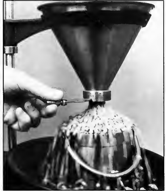
Bulk density of each sample was measured by the official test weight device approved by FGIS, USDA.
