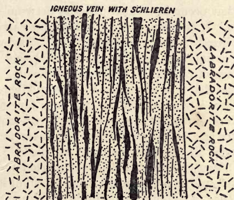
FIG. 103.—Vein of norite, 30 to 70 yd. in width with schlieren of titaniferous iron ore. (After J. H. L. Vogt.)
