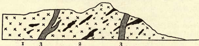
FIG. 115.—Section to illustrate the mode of occurrence of iron ores in the Ekersund—Soggedal district. (After Thomas and MacAlister's Geology of Ore Deposits .)
