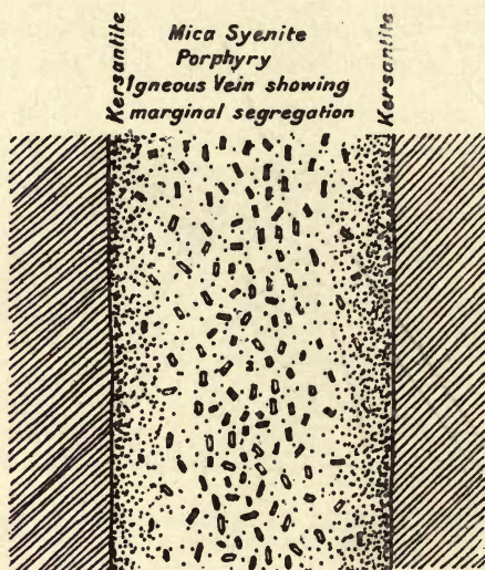
FIG. 19.—Vein of mica syenite-porphry, showing marginal segregation of ferro-magnesian minerals and iron ores. (After J. H. L. Vogt.)
