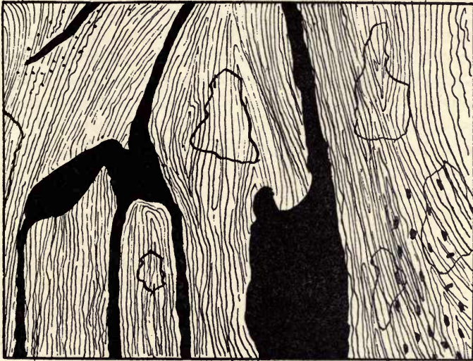
FIG. 124.—Section exposed in a pit in the Dobbins mine in Georgia. The black bands represent manganese ore and the shaded portion clays. (After Penrose.)
