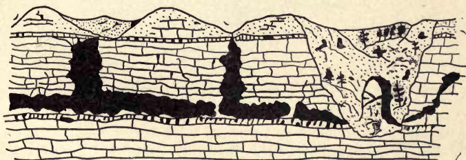
FIG. 3.—Ideal section through a limestone region showing caves left by the removal of the rock.
