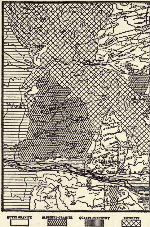
FIG. 86.—Geologic map of the western half of Butte, Montana, district. (By permission of the Macmillan Company, from Ries' Economic Geology .)
