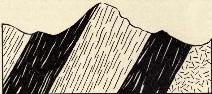
FIG. 26.—Iron ores of Michigan interbedded with igneous and sedimentary rocks. (After Emmons.)
