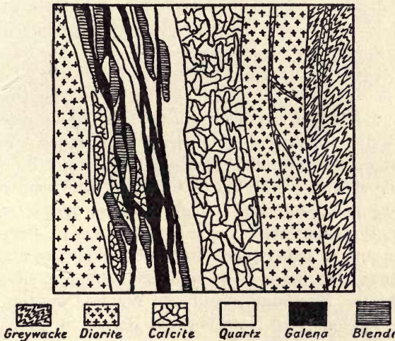
FIG. 73.—Section of the Adelbert lodes, Pribam, Bohemia. (After J. Zadrzil.)
