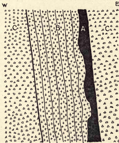
FIG. 42.—Section in the Elkton mine, Cripple Creek district, Colorado, showing the relation of the vein A to the dike B and to the country rock C . (After Penrose.)
