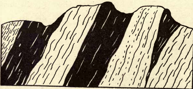
FIG. 25.—Iron ores of Michigan interbedded with sedimentary rocks. (After Emmons.)
