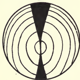
FIG. 81.—Biaxial figure for a section at right angles to an optic axis.
