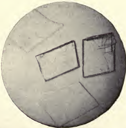
FIG. 213.—Microfragments of calcite in Canada balsam, showing strong relief due to ordinary ray (1.658), and weak relief due to extraordinary ray (1.56).
