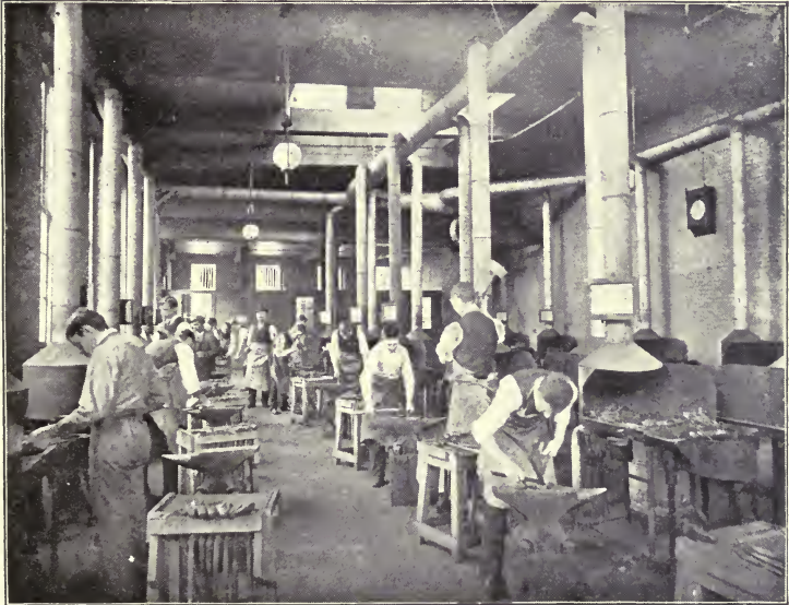
Fig. 42. Forge Shop, Overhead Exhaust Piping, Pratt Institute, Brooklyn, N. Y.
