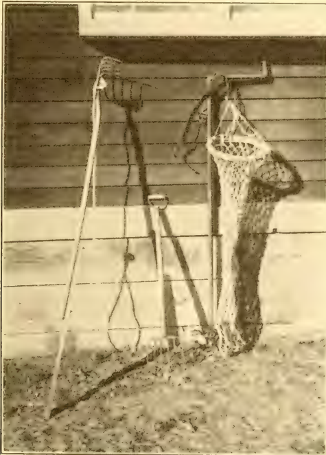
FIG. 21. Gear used in digging Pismo clams, Oceano. "Rake" with extension handle and rope by which it is pulled through sand, fork and "drag" with snap and belt.
