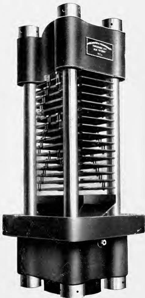
FIG. 1.—HYDRAULIC PRESS (PLATES SUPPORTED BY LINKS).
