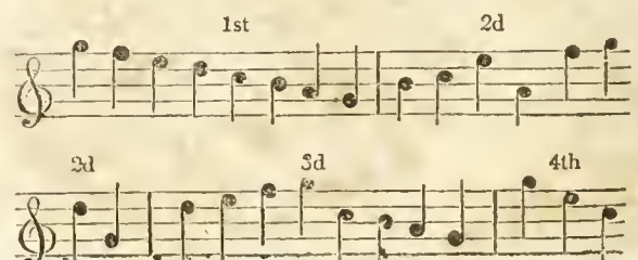
A set of Chimes for Clock Quarter Barrels, which make one revolution in an hour.
