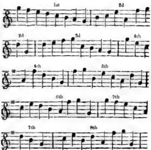
A set of Chimes for Clock Quarter Barrels, which make one revolution in an hour.
