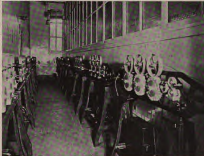
Photograph by Fox Film Company Motor-driven Felt Polishers, Through Which the Celluloid Drama Must Pass Before It Is Ready For the Projector
