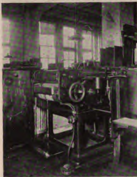
Photograph by The New York Edison Company Electric Heat Is Also Used With the Case-Making Machines Which Glue the Cloth to the Board Covers
