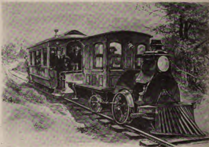
The Forerunner of Our Present Electric Locomotives. An Experimental Train Operated at Edison's Home at Menlo Park, New Jersey
