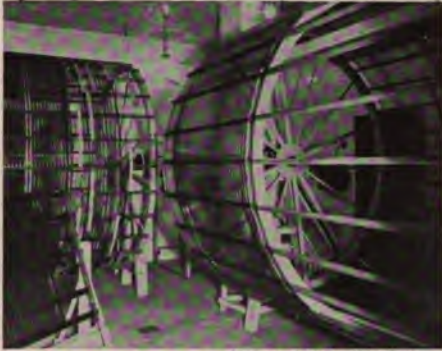
Photograph by Fox Film Company Miles of Film Wound on Drums for Drying, in Purified Air
