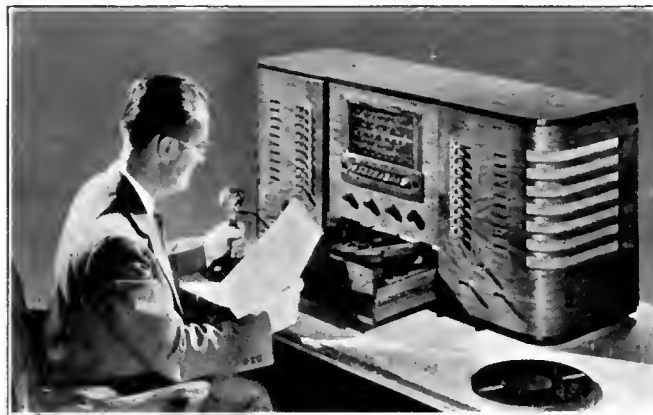
A school principal making an announcement to students in classrooms throughout his school, using the new RCA Victor "table model" sound control cabinet.
