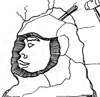
Head—entirely covered with mortar—strings withdrawn—two sections removed—note use of wedge to loosen third
