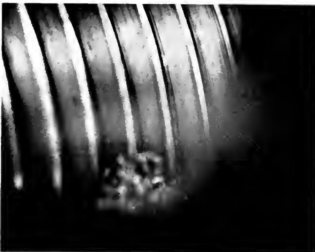
Cutting an External National Fine Thread. (One of the films on The Engine Lathe)
