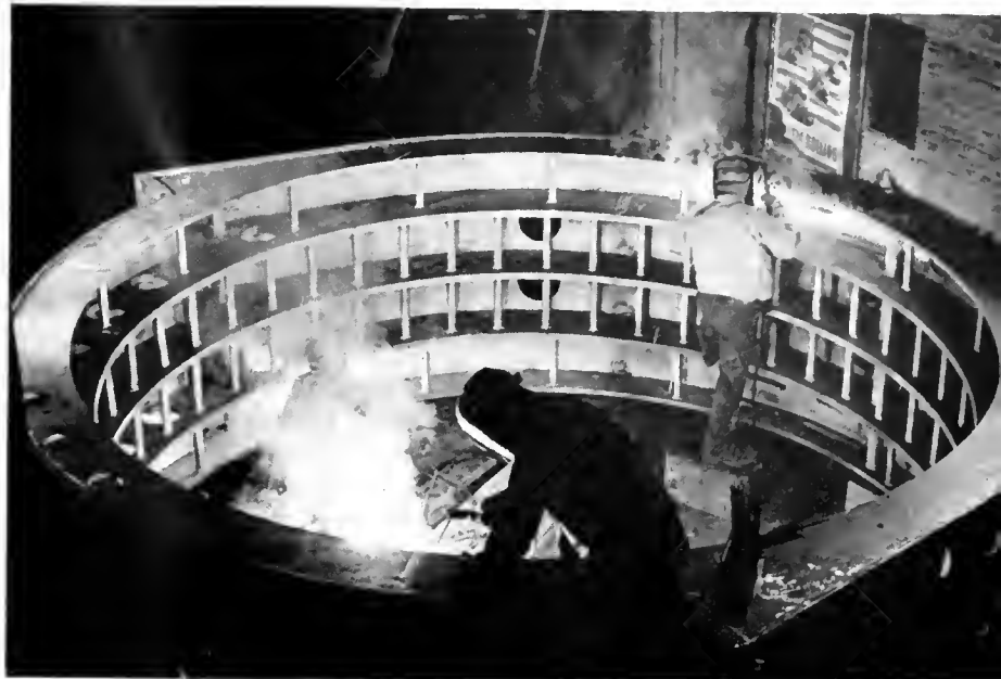
Welders working on huge motor frame, shown in the General Electric film, "The Inside of Arc Welding."
