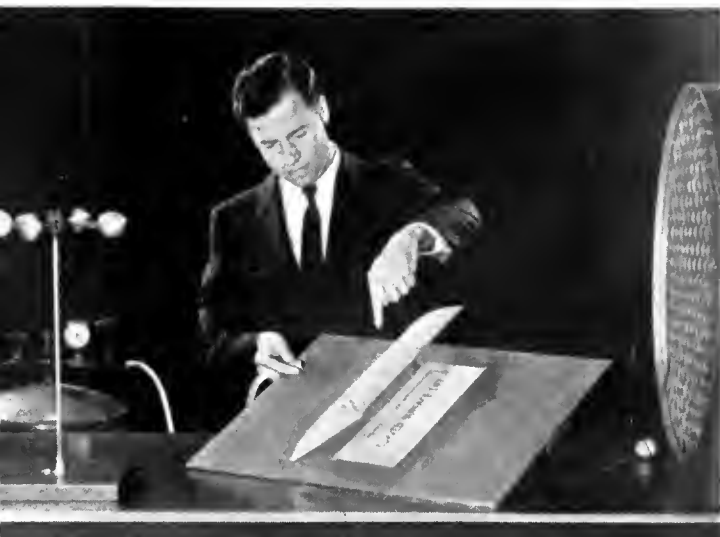
Demonstrating the effect of a swift current of air on top curved surface of plane's wing, in the Bray motion picture "Youth Takes to Wings."
