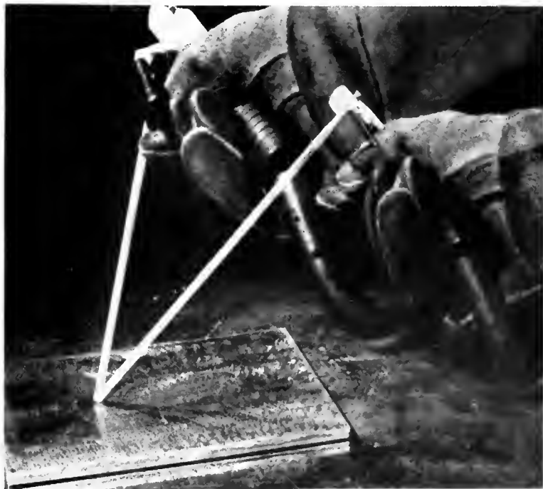
View from General Electric's "The Inside of Arc Welding," showing (left) the proper and (right) improper angle of electrode for a correct arc under normal conditions.
