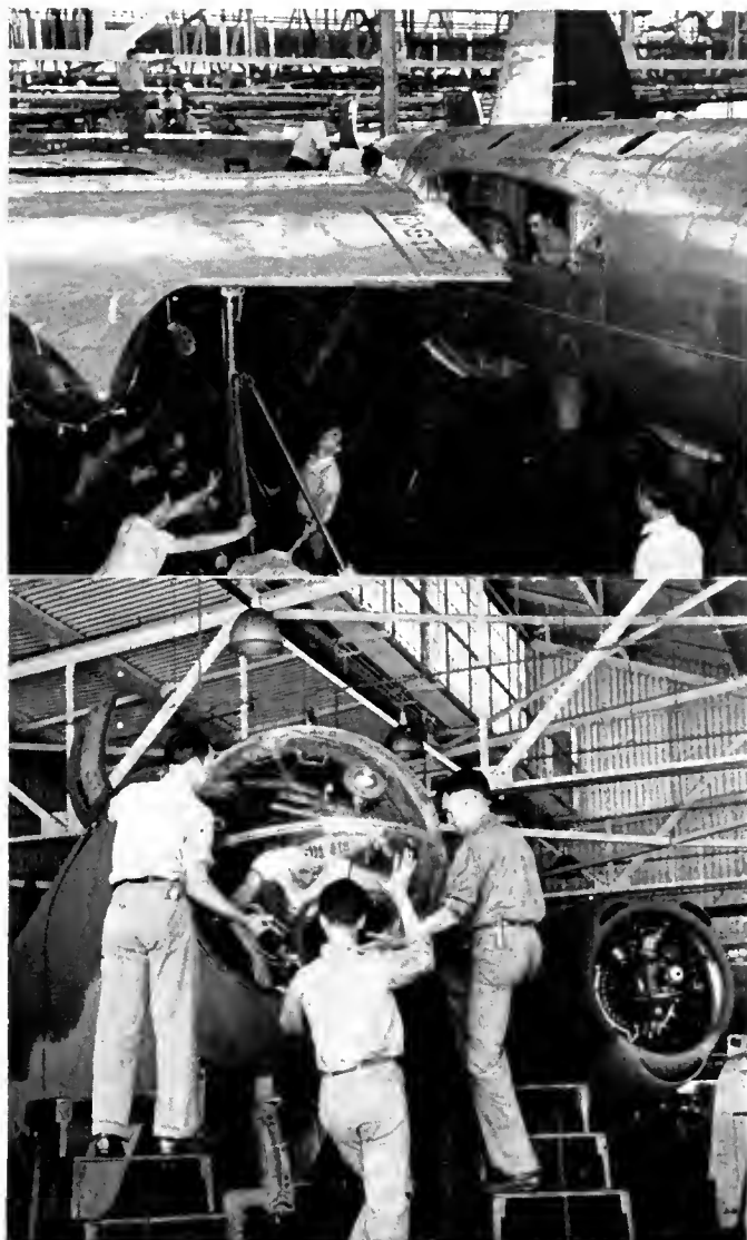
OEM Defense Photo Joining wing and nose to a Martin Army Bomber.
