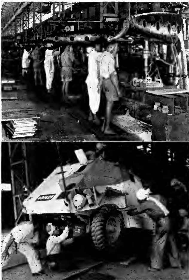
Drilling armor plate for armored carriers in Indian Railway Works, and a carrier on the assembly line. From "Made in India" (British Information Services)
