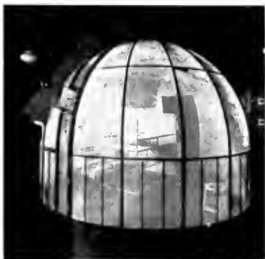
"One-way vision dome" at the Yale psycho-clinic. The wire mesh of the dome, brightly lighted within and dark outside, appears solid to the unsuspecting baby in the crib.
