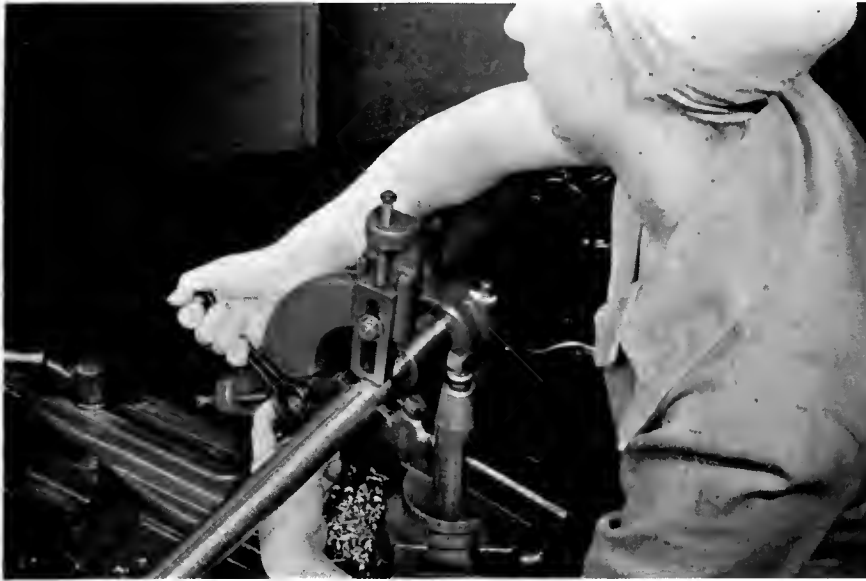
Right: Frames from the Jam Handy slidefilm unit on Mathematics. Below: From "Using a Follower Rest," one of the USOE films on the Engine Lathe, distributed by Castle Films.
