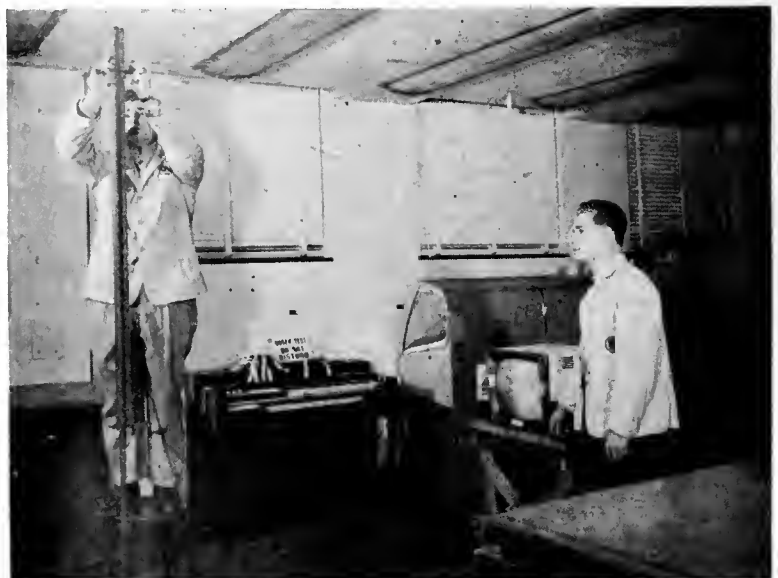
UL engineers prepare for the Impact Test on a portable TV set, to test the strength of the safety glass window protecting the picture tube. A swinging steel ball strikes the window with a force of 5 ft.-lbs. and must not penetrate into the tube.
