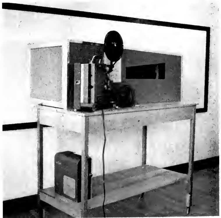
Portable table mounted on wheels, has area on top for holding a motion picture or filmstrip projector, a mounted plane mirror, a hinged screen and an enclosure to prevent undue spread of light. Shelf below, has cleats attached to hold projector loudspeaker case.
