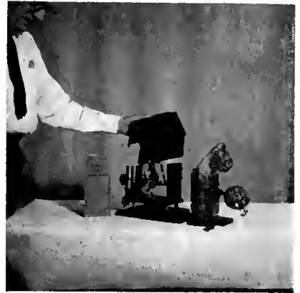
Edison Home Kinetoscope (1912, ran special 22mm film that carried three parallel rows of tiny images, the first run forward, then with lens racked over ran the second in reverse direction, and finally the third, again forward. There was a fourth lens position for showing postage-stamp size slides. A-8, A-10, A-9 shows archivist Wm. F. Kruse lifting arc lamp cover to indicate size of the unit.
