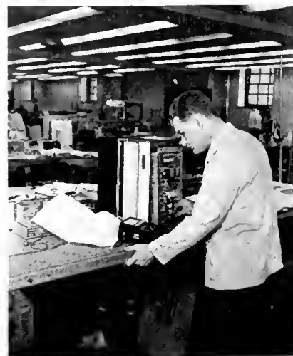
An engineer measures the maximum DC voltage at the cathode of the rectifier tube during the investigation of a tape recorder.
