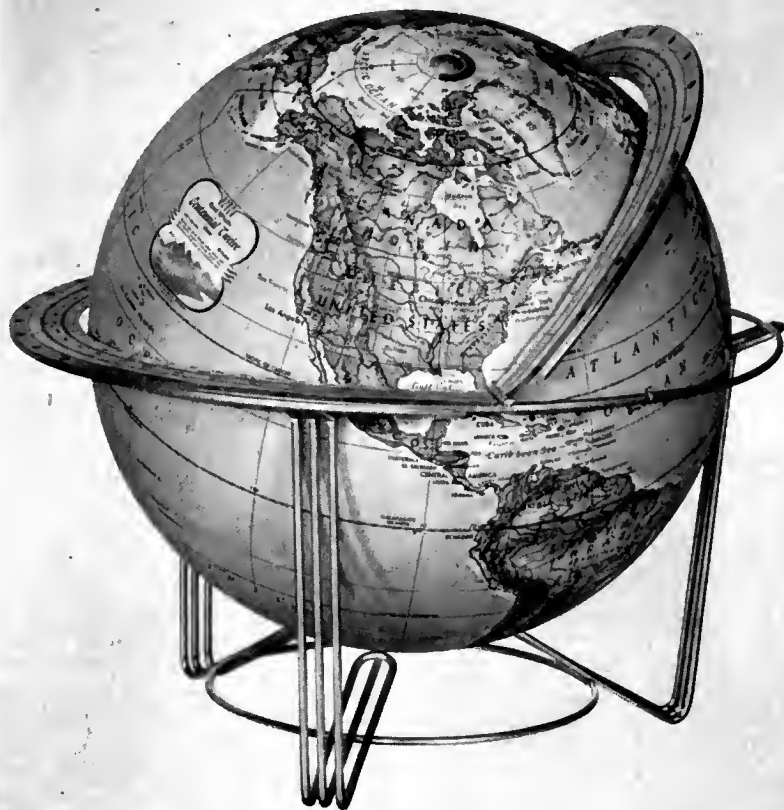
A globe equipped as a free, removable ball in a cradle horizon mounting, with a hinged great circle or satellite blade. The setting shows a great circle or rocket path from Cape Canoveral, Florida, across London, 4400 miles distance. By adjusting and rotating the globe beneath the satellite blade, the relationship of any place on earth to any satellite orbit can be visually demonstrated.
