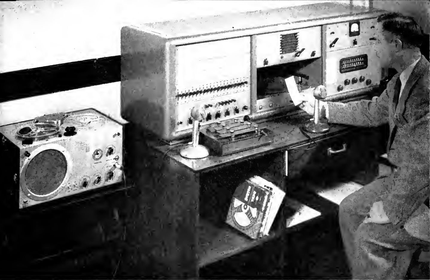
Robert L. Gregory, principal of the Theodore Roosevelt elementary school in Racine, Wisconsin, broadcasts a message to teachers and students via the school's console sound system. Chimes and the tape recorder (at left) as well as the radio and record player built into the console are important parts of the school's audio-visual equipment. (All photos courtesy Webster Electric Co.)
