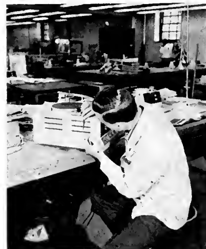
Investigating possible shock hazards, an engineer measures the ventilating openings on a phonograph to see if additional probing tests are necessary to check accessible live parts in the enclosure.
