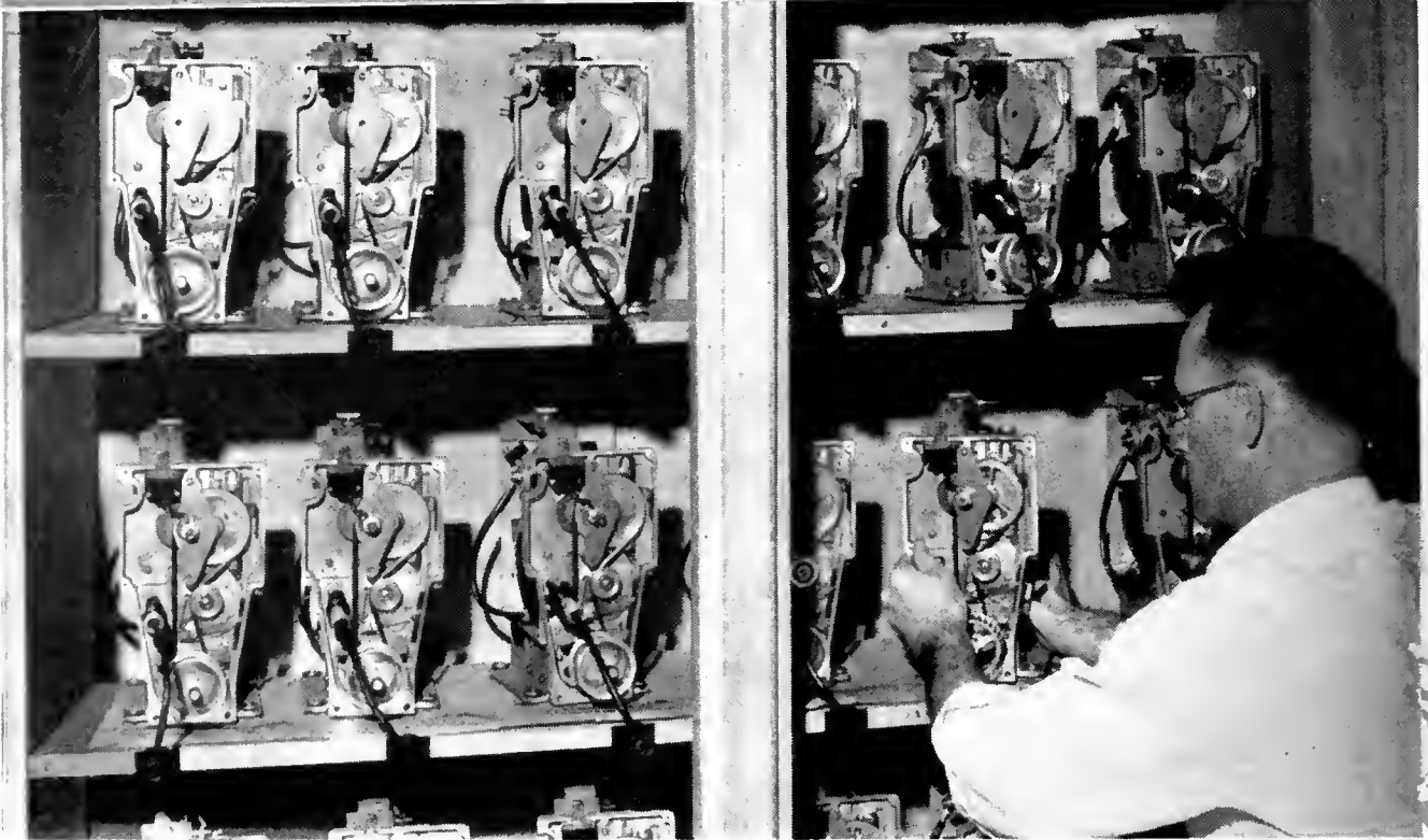
Operation of projector mechanisms in "run-in" cabinet is one of many quality controls that assures long life of Victor projectors.
