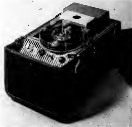
Cousino recorder with self-rewinding tape cartridge
