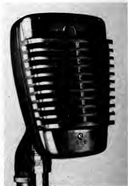
D. Unidirectional magnetic microphone, sensitive to sounds from one side
