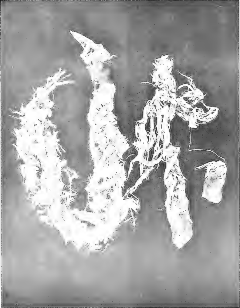
Figure 6. Cotton rope (1/2 inch diameter) fibers decayed by marine microorganisms after one year exposure.
