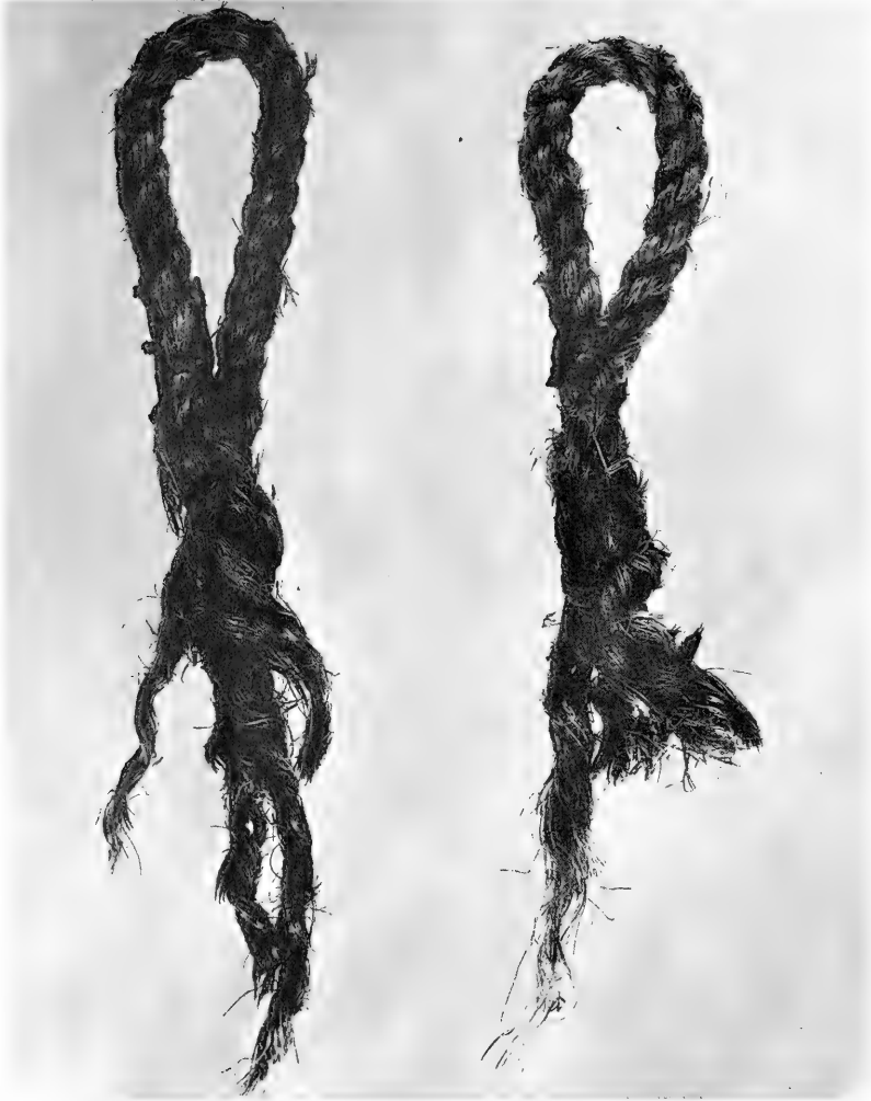
Figure 7. Manila rope (1/4 inch diameter) deteriorated by marine organisms after one year exposure.
