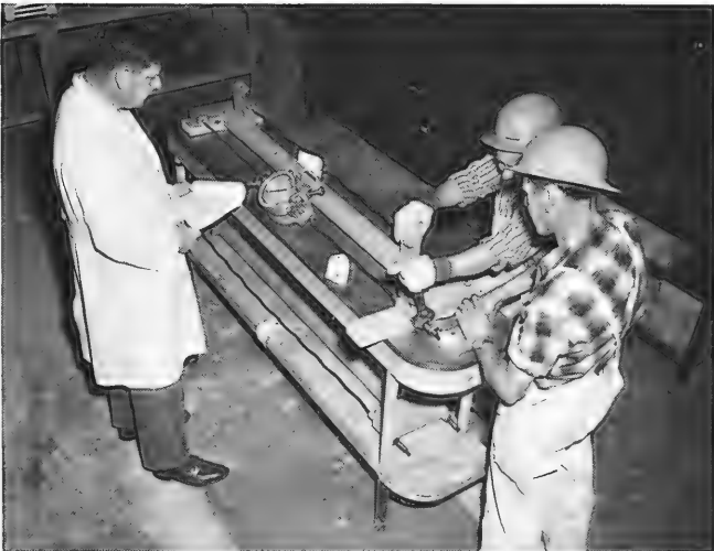
Figure 4. Cable specimen in a tensing jig being loaded to a predetermined stress level.
