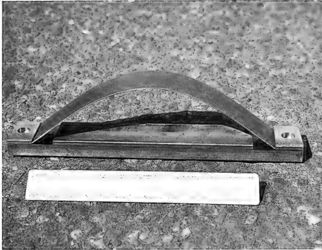
Figure 5. Stress corrosion jig with a specimen.
