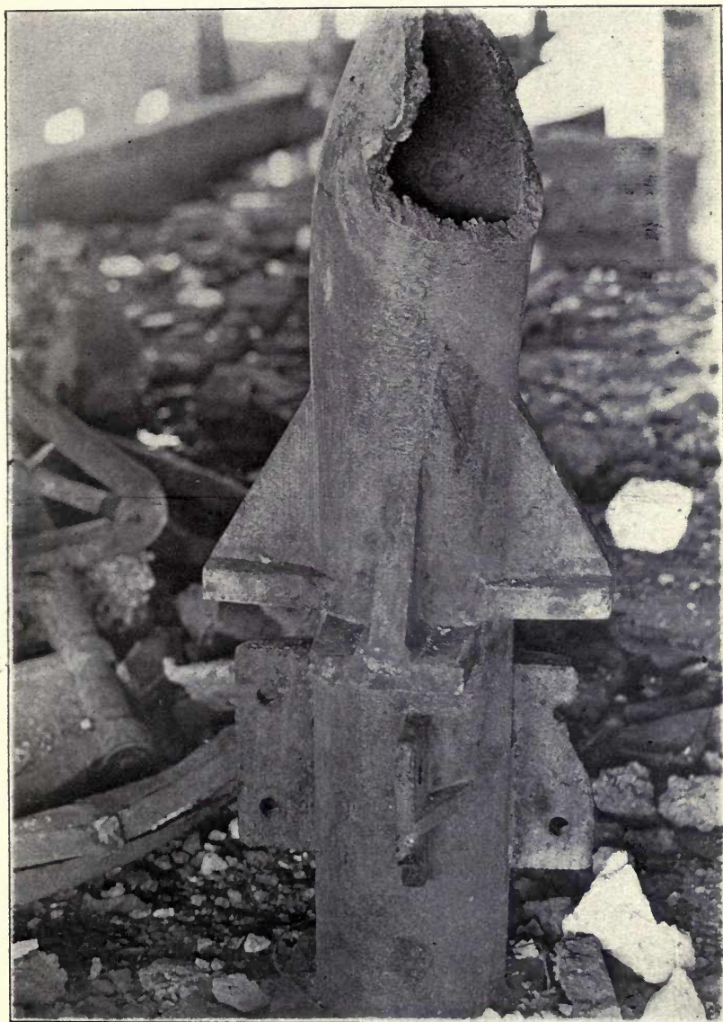
Collapsed Column (33 or 34). Eleventh Story. Showing Fracture and Effect of Heat. View Inverted.
