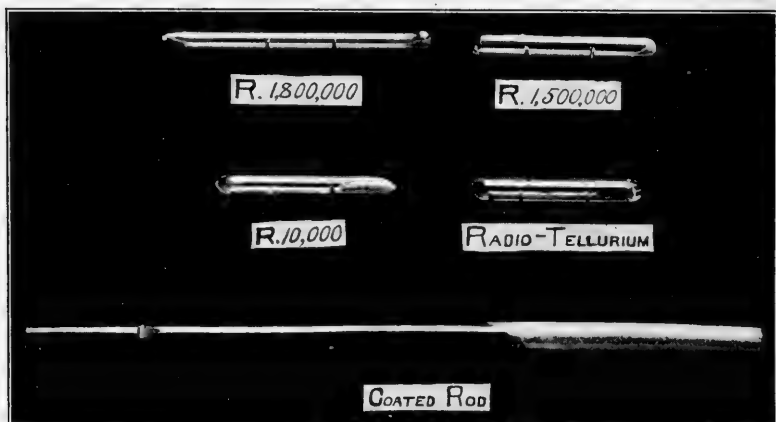
FIG. 2. Sealed Glass Tubes of Radium Bromide and a Rod Coated with Lieber's Radium Coating.
