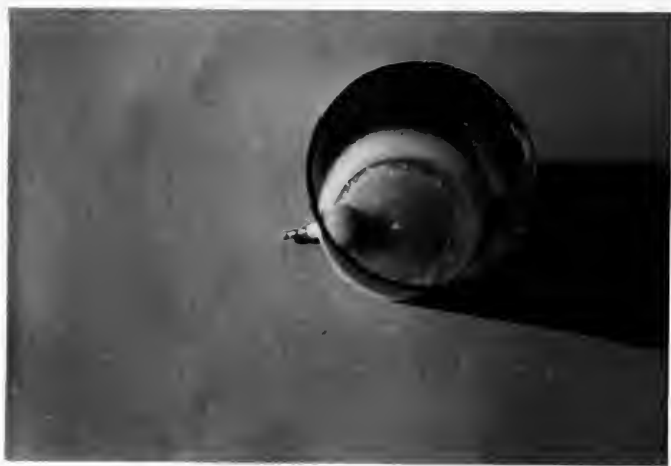
Figure 3. Sample of pots used in the experiments, with aquarium air stone in bottom to facilitate drainage and prevent sand media loss.
