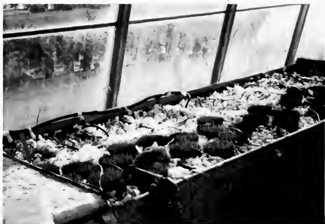
Figure 1. Experimental, compartmentalized temperature gradient plate apparatus containing four pots of grass per temperature treatment.
