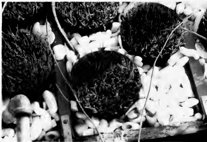
Figure 2. Pots of grass in one temperature compartment showing surface insulation used to maintain temperature levels.
