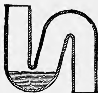
FIG. 18 represents a defective S-trap. The water does not rise above the bend and permits foul gases to get out into the room.
