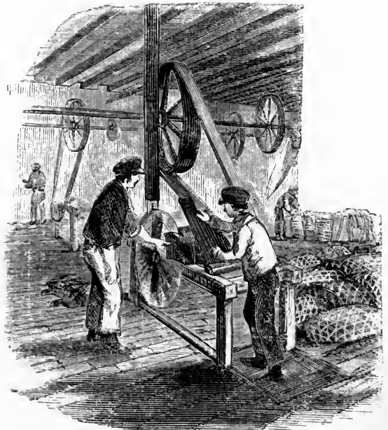
CUTTING RUBBER INTO SLABS FOR THE WASHING MACHINES.
