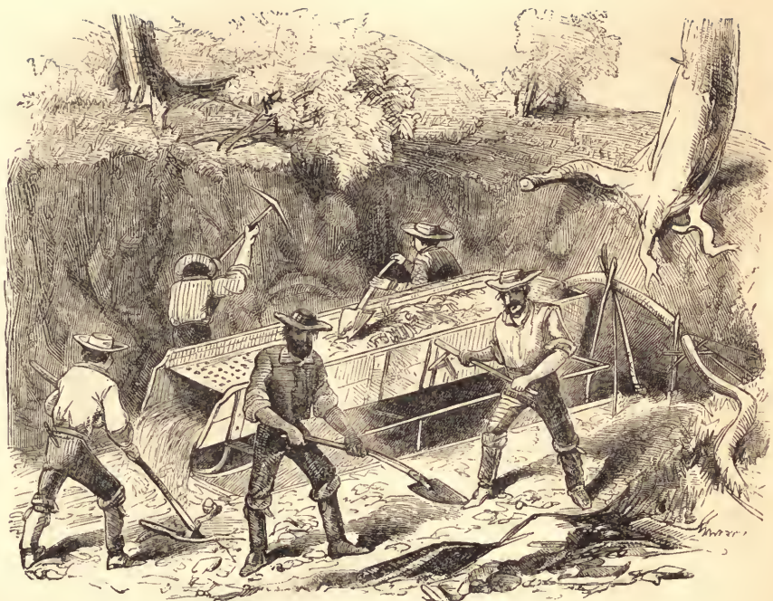
LARGE ROCKER USED IN CALIFORNIA WITH QUICKSILVER.
