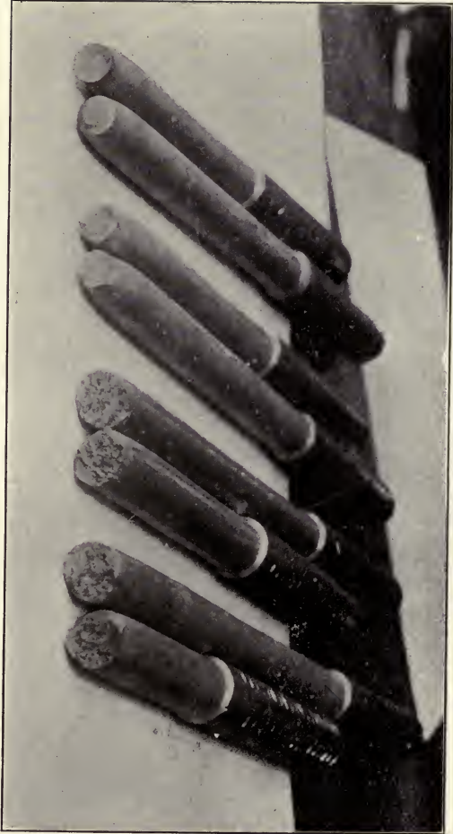
Tensile-test specimens of steel and wrought iron broken in the testing laboratory of the Department of Civil Engineering of Columbia University. The four steel specimens on the left show the characteristic "cupping" fracture. The four specimens on the right are of wrought iron and show the characteristic fibrous fracture of that material.
