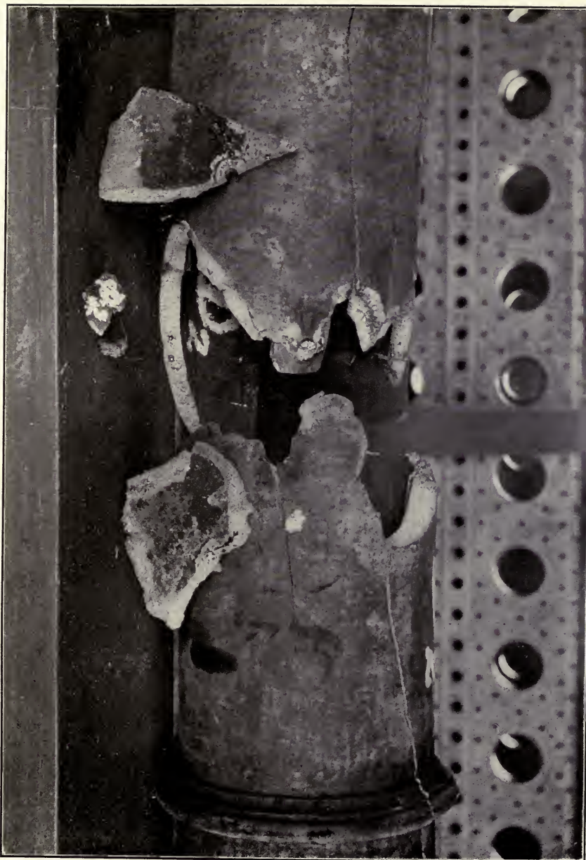
View of failure of a cast-iron column tested in the 1000-ton testing-machine of the Phoenix Iron Co. at Phoenixville, Pa.
