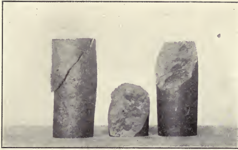
Failure of short cylinders of cast iron showing the shearing of the metal on the plane of maximum shear.
