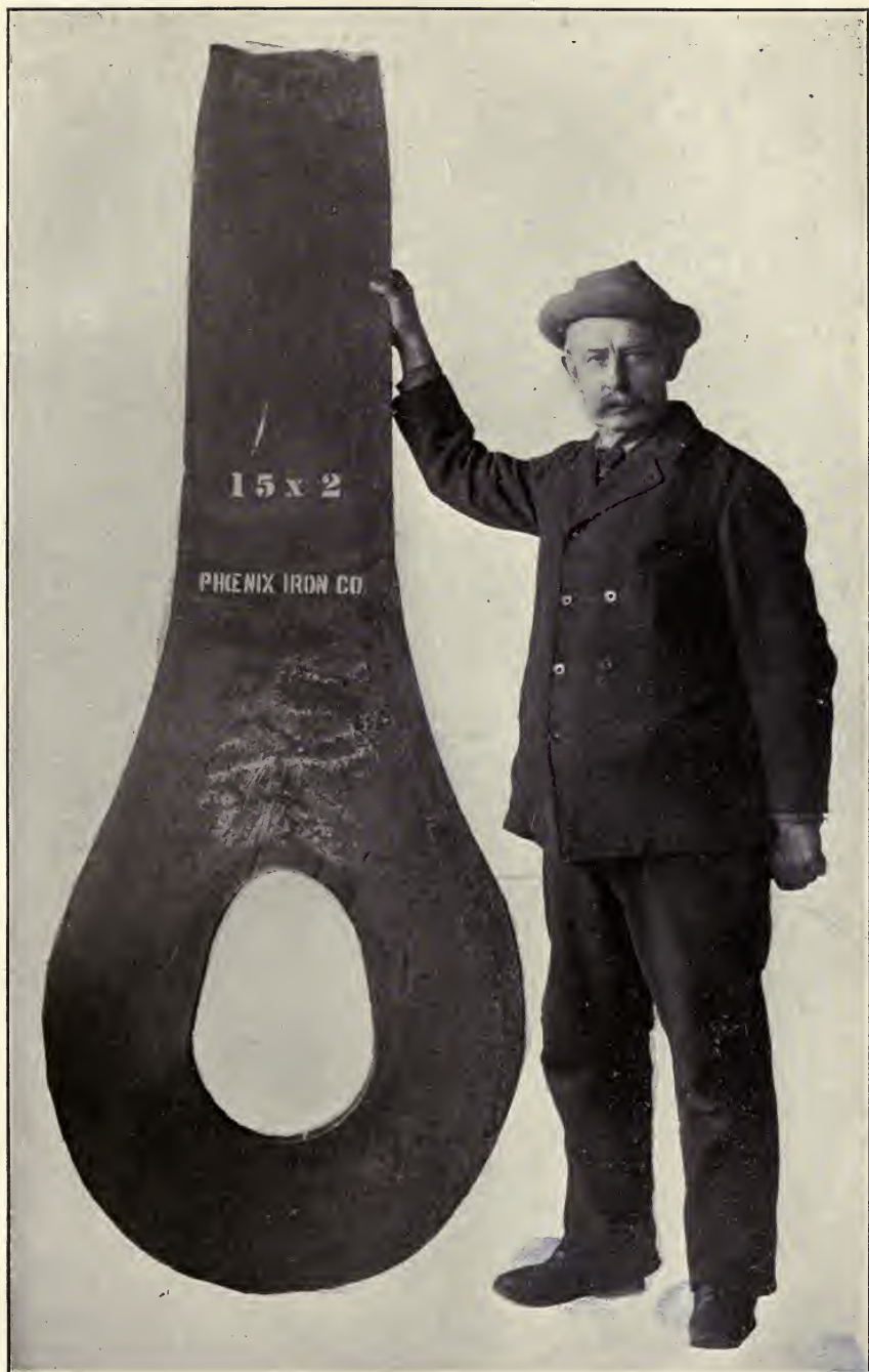
A 15 \times 2 -in. steel eye-bar forged at the shops of the Phoenix Bridge Co., Phoenixville, Pa. The bar developed an ultimate resistance of 50,160 lbs. per sq. in. and 28,000 lbs. per sq. in. at elastic limit. The elongation in 8 ins. of the bar, including the section of failure, was 25.6 per cent. and the elongation of the pin-hole was 5.26 inches. The reduction of area at the section of fracture was 52.9 per cent.
