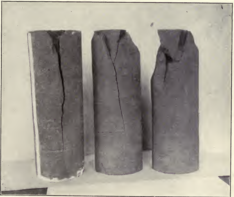
View exhibiting the failure of short cylinders of Connecticut brown sandstone. (To face page 386.)
