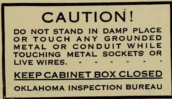
FIG 49—SAMPLES OF STICKERS PASTED ON FUSE CABINET BOXES TO GIVE EVIDENCE OF PREVIOUS INSPECTION
