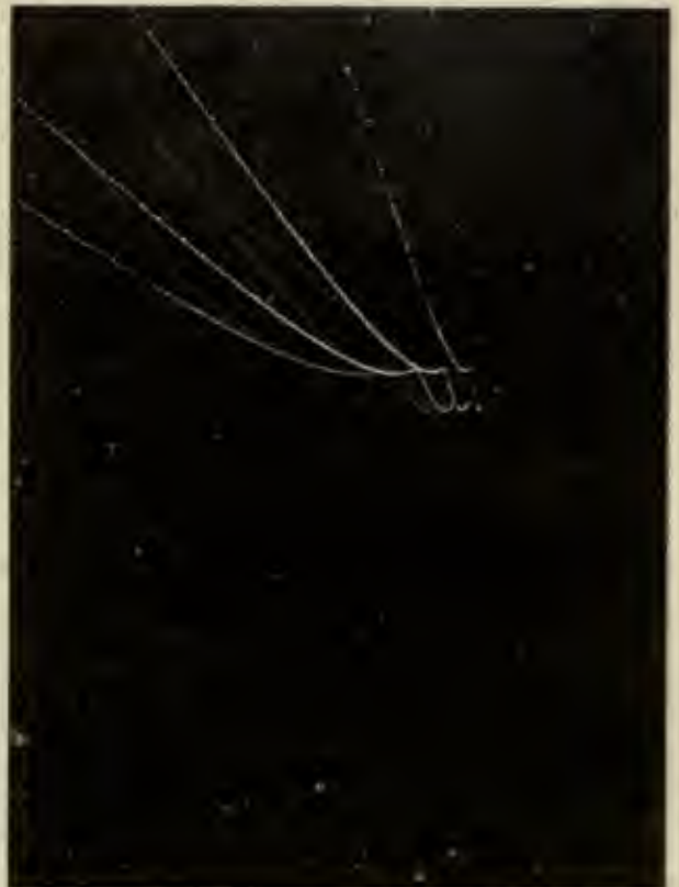
CORONA AT 230 KV. 1.19 CM. DIAMETER, 0.47" CABLE, 310 CM. 10 FEET SPACING.
