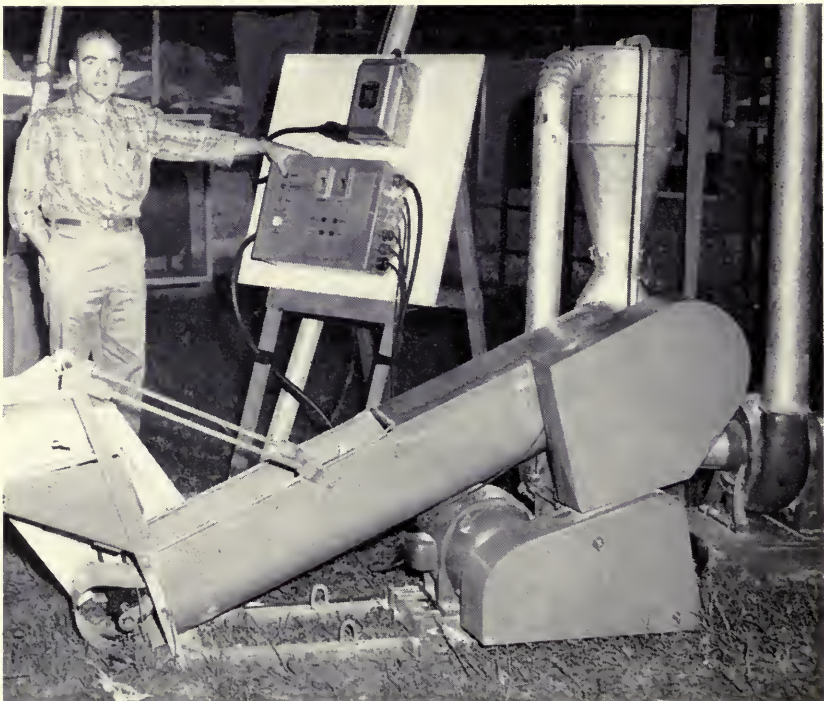
Equipment used in automatic feed grinding consists primarily of a grinder, a system of conveyors, and usually a blower to handle the ground feed. (Fig. 1)
