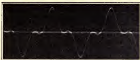
FIG. 106. Transformer voltage with Y-connection and insulated neutral.
