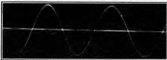
FIG. 105. Transformer voltage with delta-connected transformers or Y-connected transformers with neutral brought to generator.
