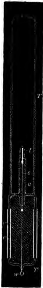
FIG. 34.—Tube with Filament Rendered Incandescent in an Electrostatic Field.
