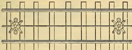
FIG. 102. Track Equipped for Track Return Circuit.
