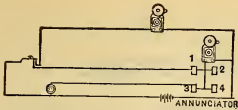
FIG. 43. Four Indication Annunciator, with extra Bell to ring from one Push only. Illustrating use of three-point button.
