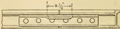
FIG. 50. Short thick Bond applied to "Tram" of Girder Rail, allowing constant inspection.
