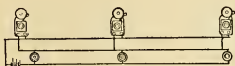
FIG. 35. Three-line Factory Call. A number of Bells operated by any number of pushes. All bells rung by each push.
