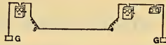
FIG. 44. Acoustic Telephone with Magneto Bell Return Call. Extension Bell at one end of line.
