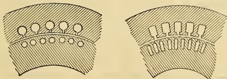
FIGS. 73 and 74. Forms of Punchings of Induction Motors.
