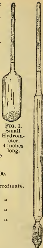
FIG. 2. Standard Hydrometer. 8 3/4 inches long.
