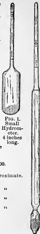
FIG. 2. Standard Hydrometer. 8 3/8 inches long.
