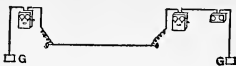
FIG. 44. Acoustic Telephone with Magneto Bell Return Call. Extension Bell at one end of line.
