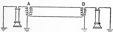
FIG. 29. Two distant grounded circuits connected through repeating coils A and B to a long-distance metallic circuit.
