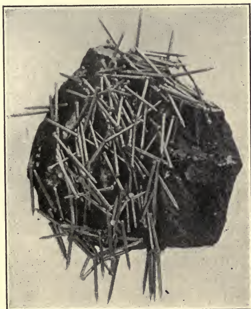
FIG. 3.—Natural magnet attracting iron nails.
