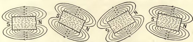
FIG. 19.—Results of breaking bar magnet in a number of parts.
