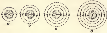
FIG. 26.—Illustrates how field builds up about a conductor as current increases.
