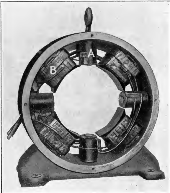
FIG. 255.—Four-pole interpole motor; one interpole for each main pole.
