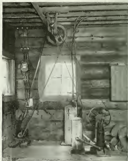
Fig. 2.—Shannon Bros.' 5 h.p. equipment for milking machine.
