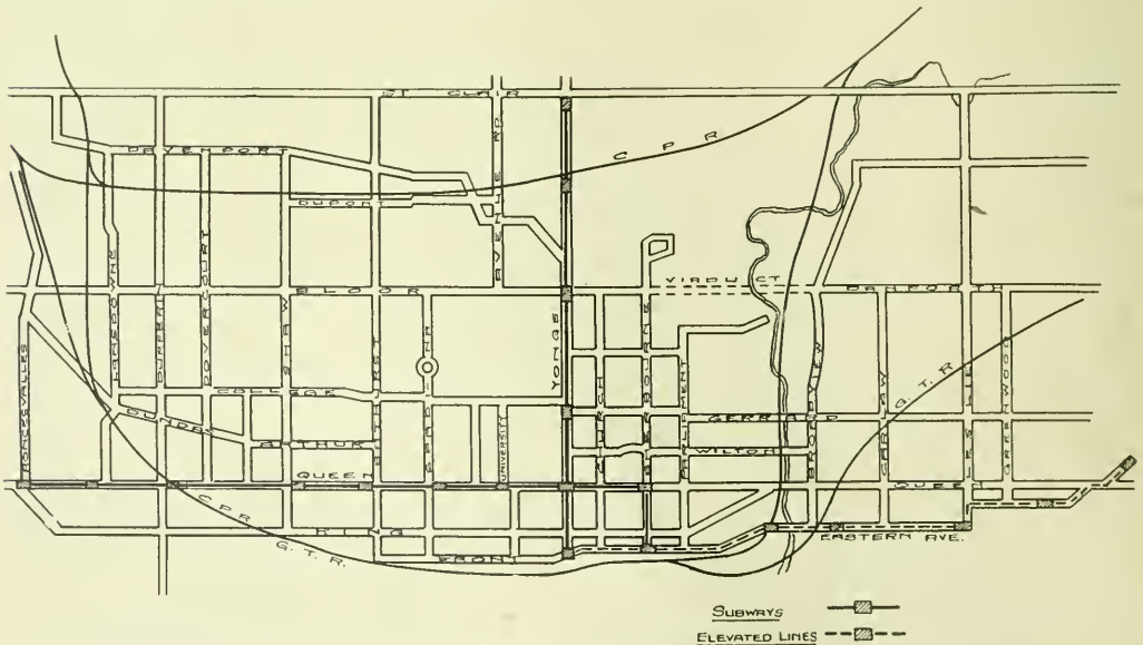
Fig. 1.—Plan of the City of Toronto showing the main streets upon which car tracks are situated and the location of the Rapid Transit Lines.
