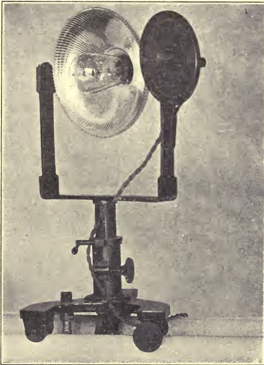
FIG. 335.—Lamp-Holder for Spherical Measurements.
