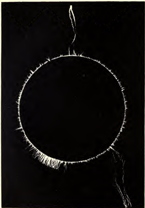
[From a photograph taken in the Cavendish Laboratory of a plate of glass with a circular tinfoil coating on one side, a larger coating being applied to the other side of the glass. The electrification of the coatings was produced by an induction coil.]
