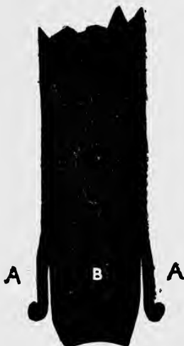
FIG. 2. —Section of Positive Carbon with the Outer Crust curling away from it.
