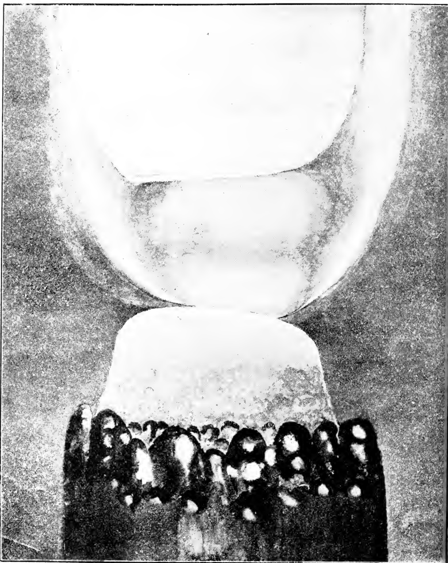
FIG. 5. —Carbons: Positive, 18mm. cored; Negative, 15mm. solid. Current, 20 amperes. P.D. between Carbons, 51 volts. Length of Arc, 7mm.
