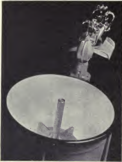
FIG. 108.—Interior view, showing agitator, of washing machine illustrated in Fig. 107
