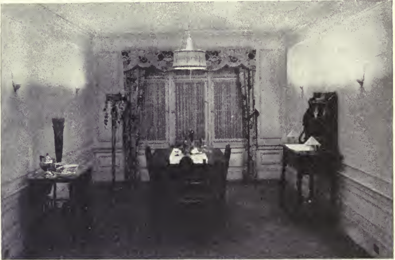
FIG. 59.—Use of center light and bracket fixtures for dining room lighting
