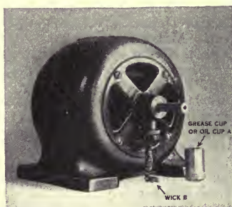
Grease or oil cup removed from motor and wick exposed
