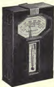
FIG. 131.—"Humidiguide" for registering relative humidity and temperature
