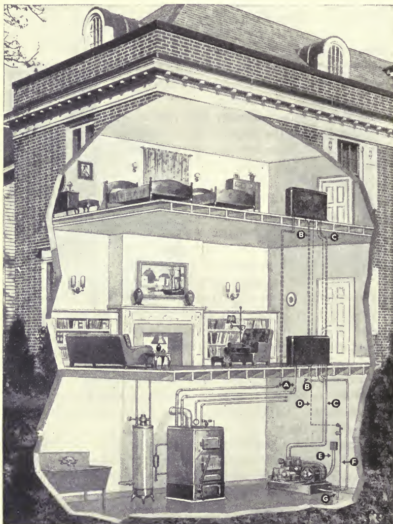
FIG. 132.—Combined air heating and cooling system installed in the home. Cooling unit in basement at right. (Letters refer to piping connections)
