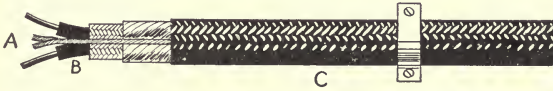
FIG. 278.—Non-metallic sheathed cable "A"—Conductors or "electric highway" "B"—Electrical insulation "C"—External protective covering
