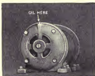
FIG. 101.—Parts of the motor that require lubrication. Wick "B" in center illustration conducts oil or light grease to motor bearing
