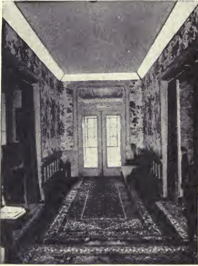
FIG. 38.—An example of architectural lighting bordering the ceiling
