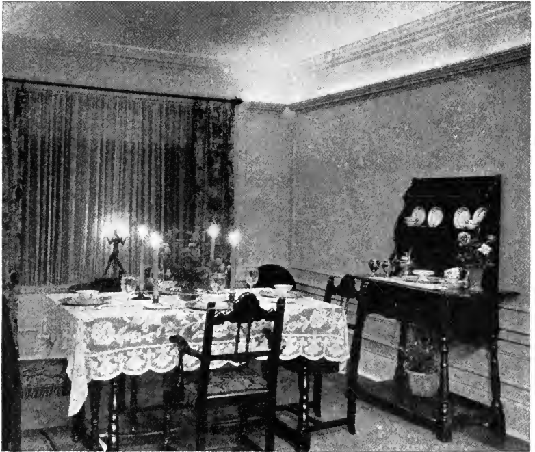
FIG. 34.—An example of cove lighting bordering the ceiling
