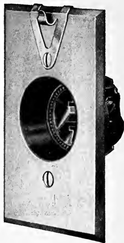
FIG. 17.—A special outlet for a wall clock, provides a hook and requires a short connecting cord. With hook removed it has other uses
