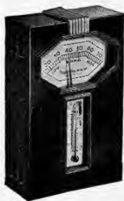
FIG. 131.—"Humidiguide" for registering relative humidity and temperature
