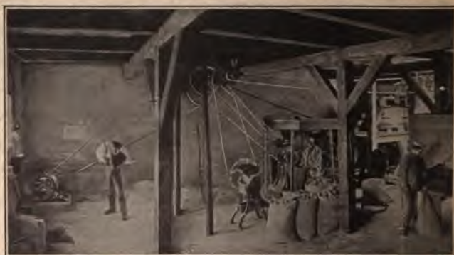
Fig. 23. Electric-operated grain mill on a large farm. A single motor drives a group of machines.
