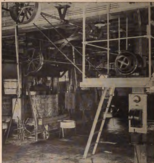
Fig. 21. Fruit press operated by stationary motor to make farm by-products.
