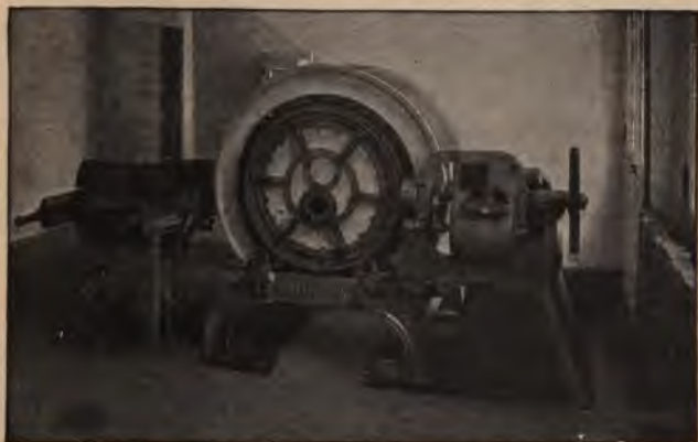
Fig. 17, Butter churn operated by direct geared motor.
