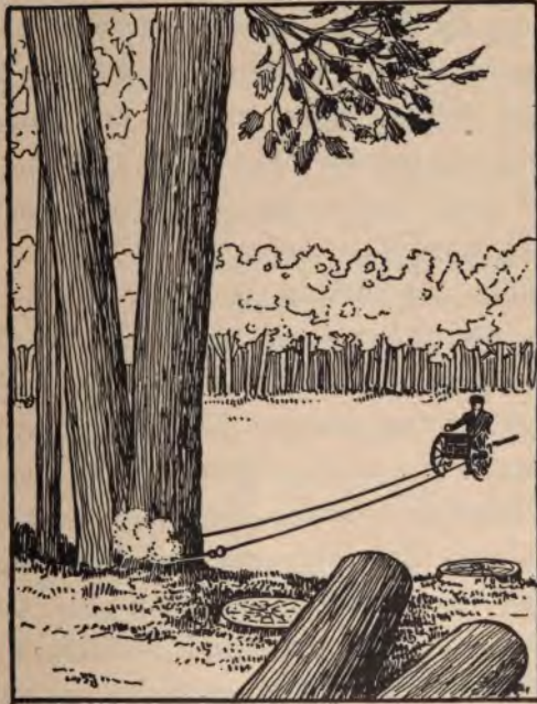
Fig. 39. Apparatus for felling trees by electricity.
