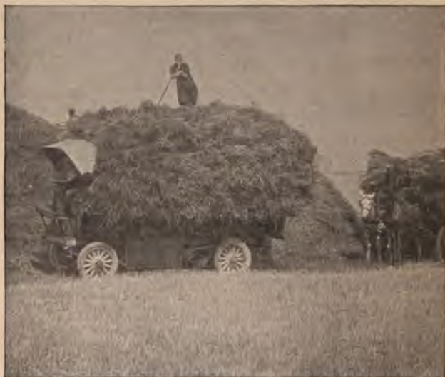
Fig. 28. A 3½ ton electric truck carrying 617 bundles of wheat. Electric vehicles carry three times the load of horse-drawn vehicles and dispense with one farm hand.
