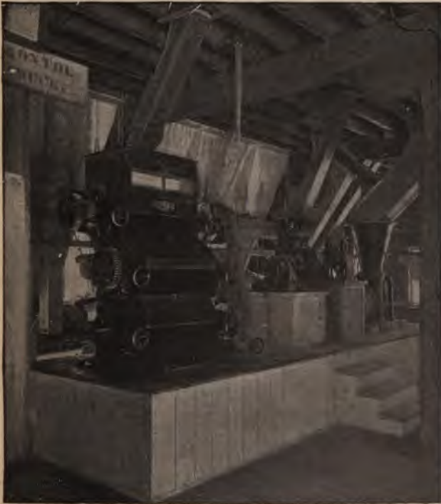
Fig. 22. Grist mill machinery on a New York farm, operated by portable motor.
