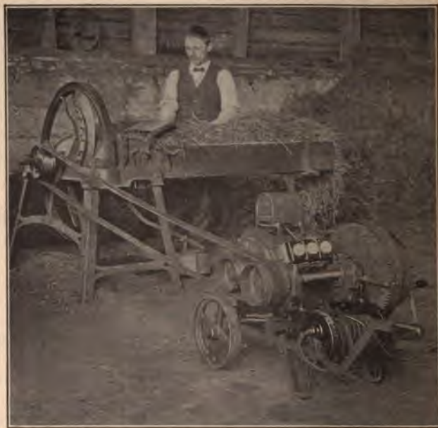
Fig. 14. Hay cutter operated by portable motor, equipped with three different sizes of pulleys, suitable for different speeds of driven machinery.
